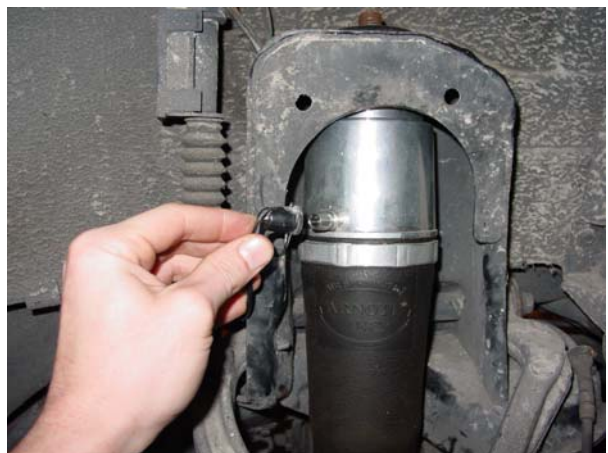
13. Clip air hose back on air shock fitting. ↑
