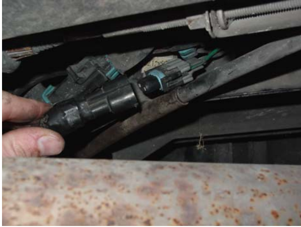
7. Unplug strut damper solenoid, and remove cable from mounting brackets. ↑
