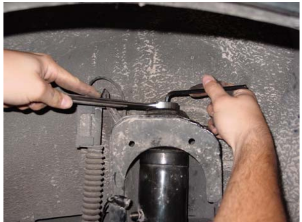
6. Remove upper nut, retainer, and insulator ↑
