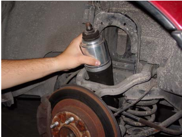
9. Position top of shock absorber with insulator and install through upper control arm. ↑
