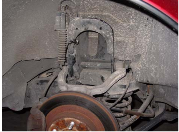
8. Compress shock and remove through ↑ upper control arm.
