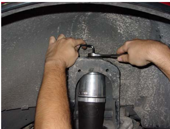
11. Replace upper shock absorber insulator, retainer, and nut. ↑
