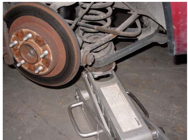
4. Support lower control arm with floor jack to relieve spring load. ↑
