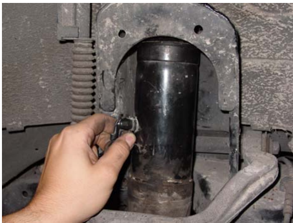
3. Remove air line by rotating steel clip. ↑
