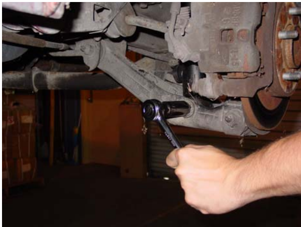
5. Remove lower nut and bolt. ↑
